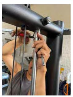
**Step 5**Lift off the top plate and cable attached assembly.
